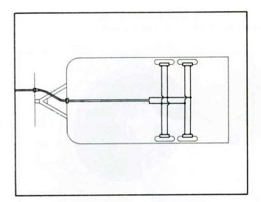
Brakes must be wired in parallel and good quality insulated crimp type connectors should be used.
