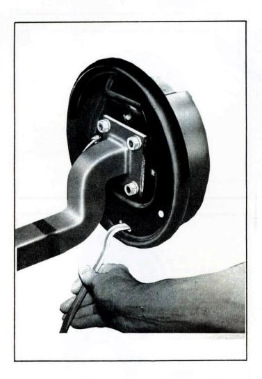
5. Brakes are pre-adjusted at the factory and normally do not require additional adjustment when mated with new drums. The drum should be checked for freedom of rotation after mounting and the brake re-adjusted if dragging occurs. Brakes should be checked for proper alignment if mated with used drums.
