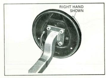
The brake is mounted on the axle flange with the magnet located towards the bottom of the brake.
