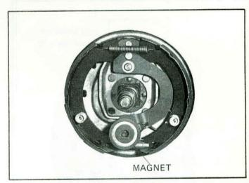
3. Tighten mounting nuts evenly with 75 to 80 foot lbs. torque. Be sure the pilot hole in the backing plate mates properly with the pilot on the axle flange so that the brake assembly is square when secured in place.
